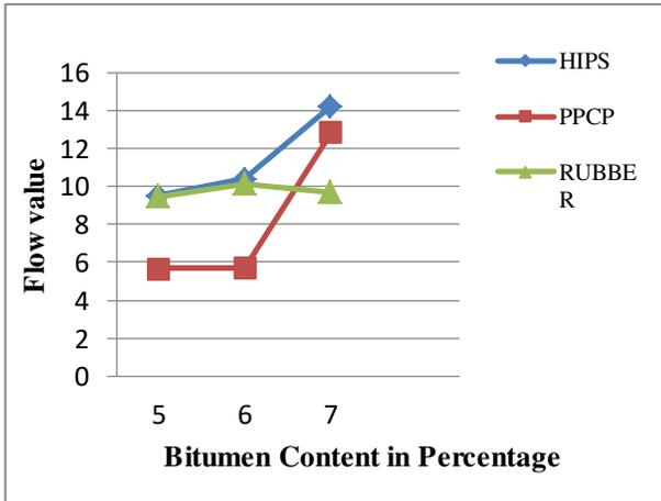
Fig. 3 Bitumen content vs Flow value
