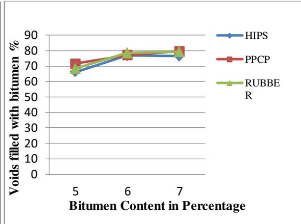
Fig. 4 Bitumen content vs VFB
