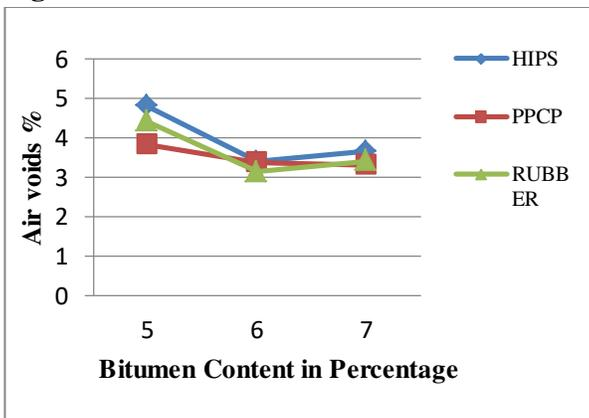
Fig. 5 Bitumen content vs Air voids
