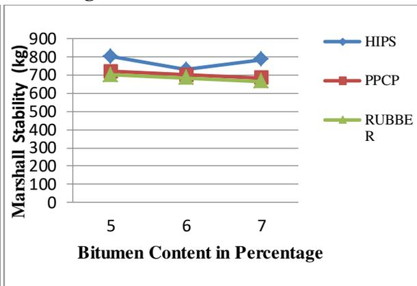
Fig. 6 Bitumen content vs Marshall Stability
